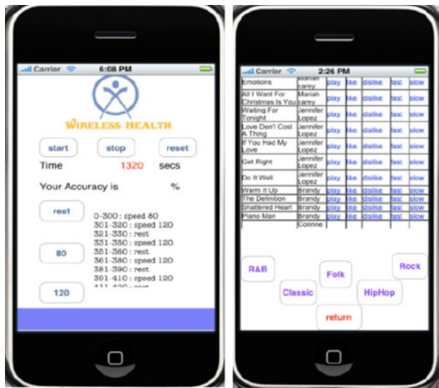
Fig. 5 A customized interval training system. This system uses accelerometer functionality, GPS, graphical, sound, vibration, etc. functionalities on an iPhone
