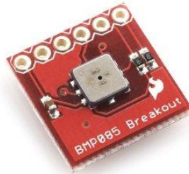
Figure 4.9 BMP085 Barometer Board.
