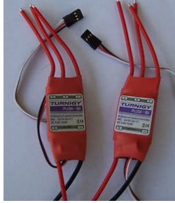
Figure 4.3 Turnigy Plush18A ESC Packs.
