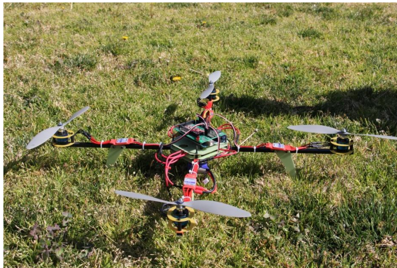
Figure 4.13 Quad Copter As Constructed.
