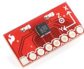
Figure 4.8 BMA180 Accelerometer Board.
