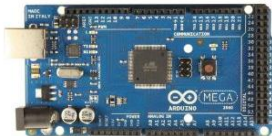
Figure 4.1 Arduino Mega 2560 Microcontroller Board.
