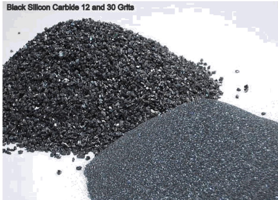
Figure 2.3 Black Silicon Carbide Abrasive Grains
