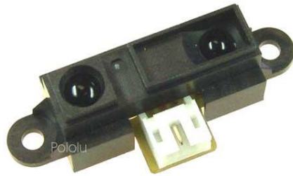
Figure 5.3- SHARP Infrared Proximity Sensor
