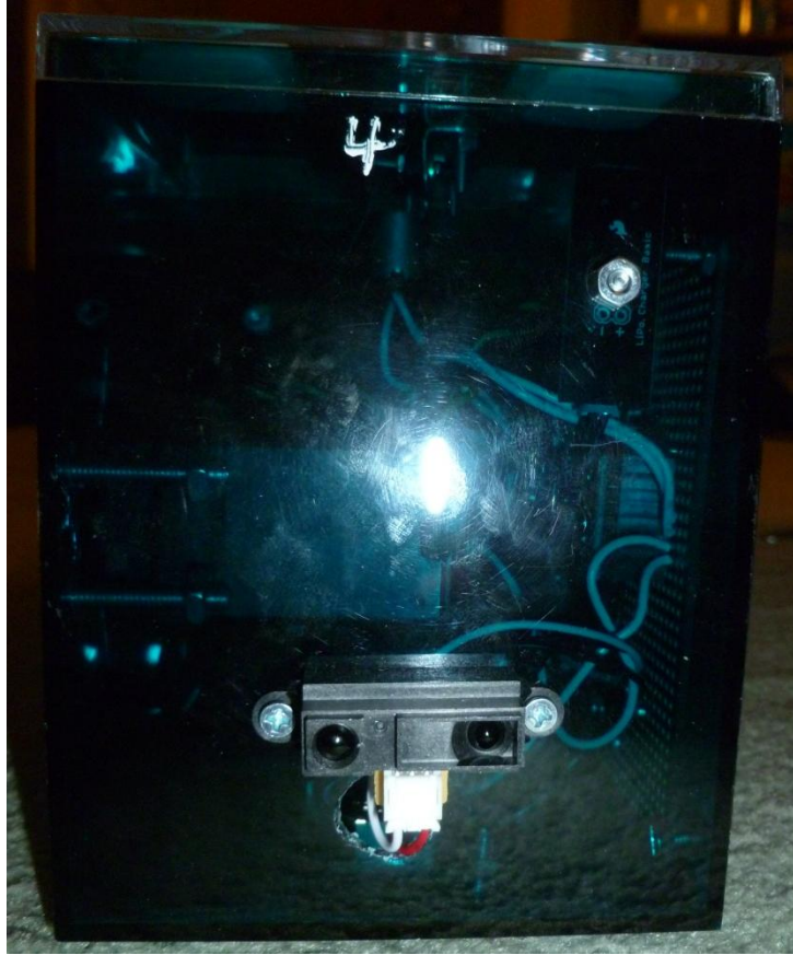
Figure 8.8- Side of Box with IR Distance Sensor
