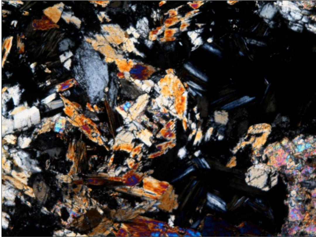
Figure C-9. Thin-section of SDI-8538 Soapstone Type 1 (Talc, chlorite, coarse-grained).
