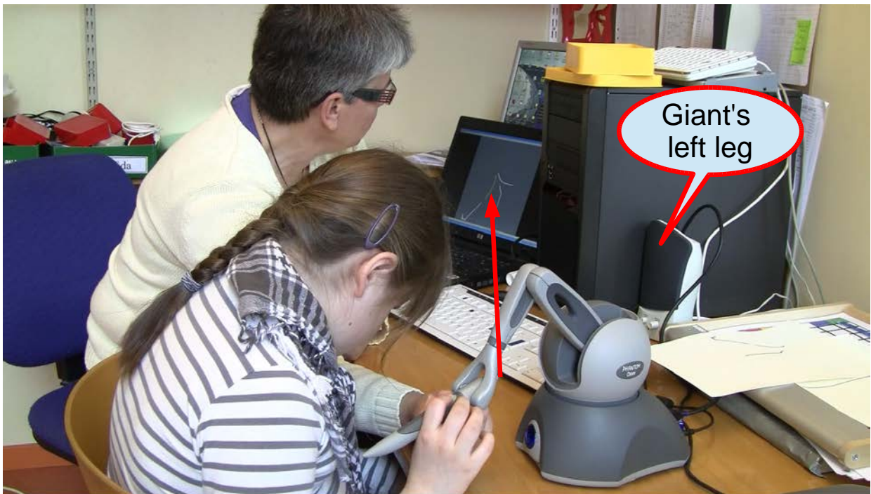
Fig. 1. HIPP Concept Picture. The pen for haptic feedback of the drawing on screen, the speaker for spoken feedback or sound effects related to the point the pen is touching.
