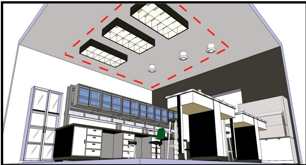
Figure 4.14 Proposed design with combined fluorescent and LED lamps (numbers of fixtures will be determined based on appropriate load and lighting density calculations)
