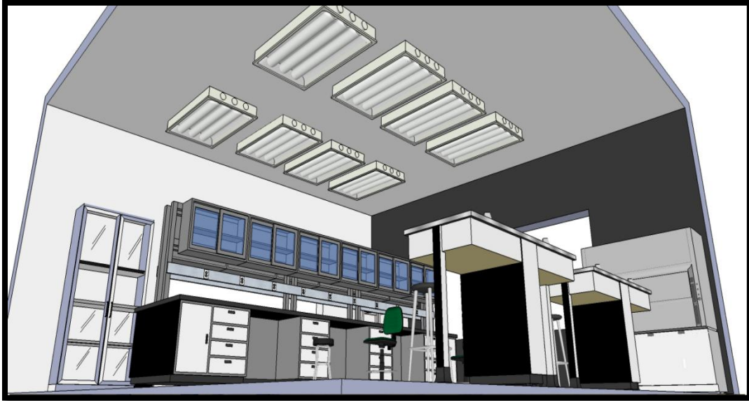
Figure 4.13 Existing ceiling design with full size fluorescent lamps
