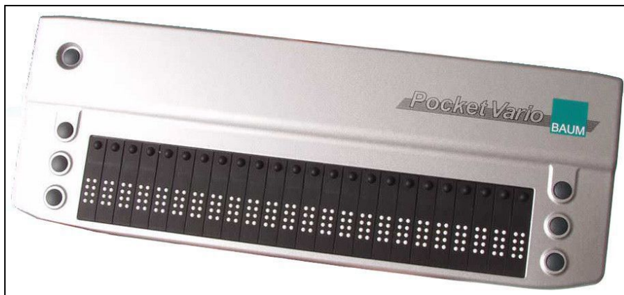
Figure 2-1. A Braille Display. A typical 8-dot Braille display with 24 Braille cells. Six buttons on either side of the board are used for typing. Braille displays like this cost between $500 and $3000.
