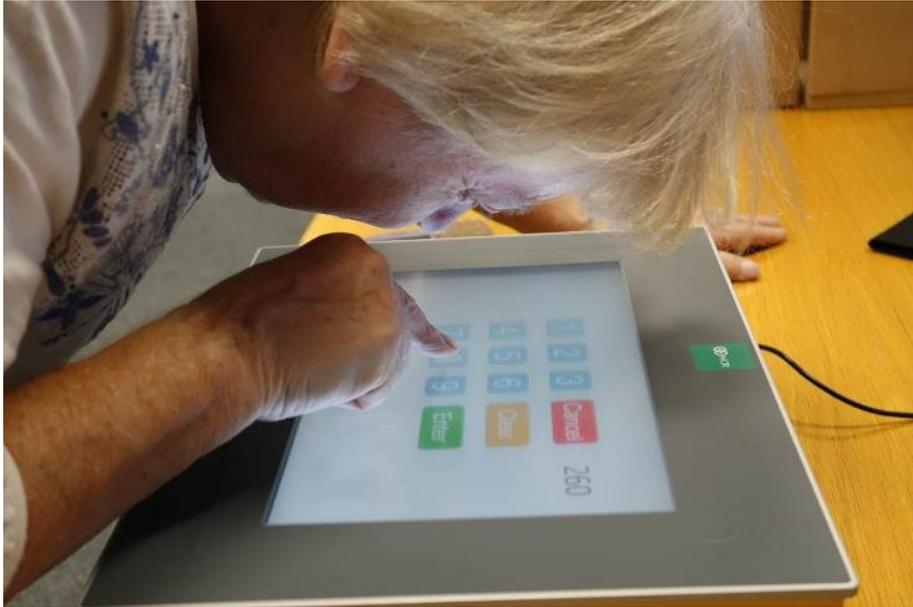
Fig. 10. Concept 3 for PIN entry: Haptic touchscreen.
