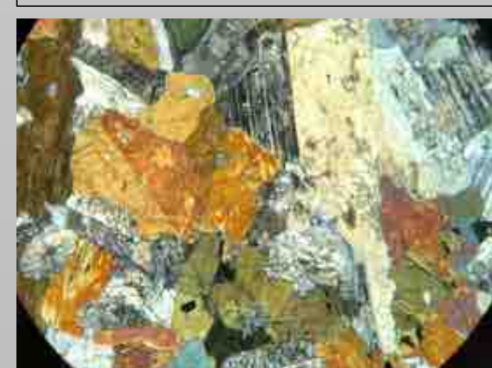
1. Plagioclase 2. Hornblende 3. Perthitic Texture 4. Orthopyroxene? 5. Clinopyroxene? (XPL) Magnification: 40x.
