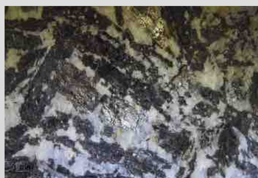
Photographs showing phaneritic texture dominated by elongate hornblende crystals in a matrix of plagioclase with green deposits of epidote or olivine visible in close up.
