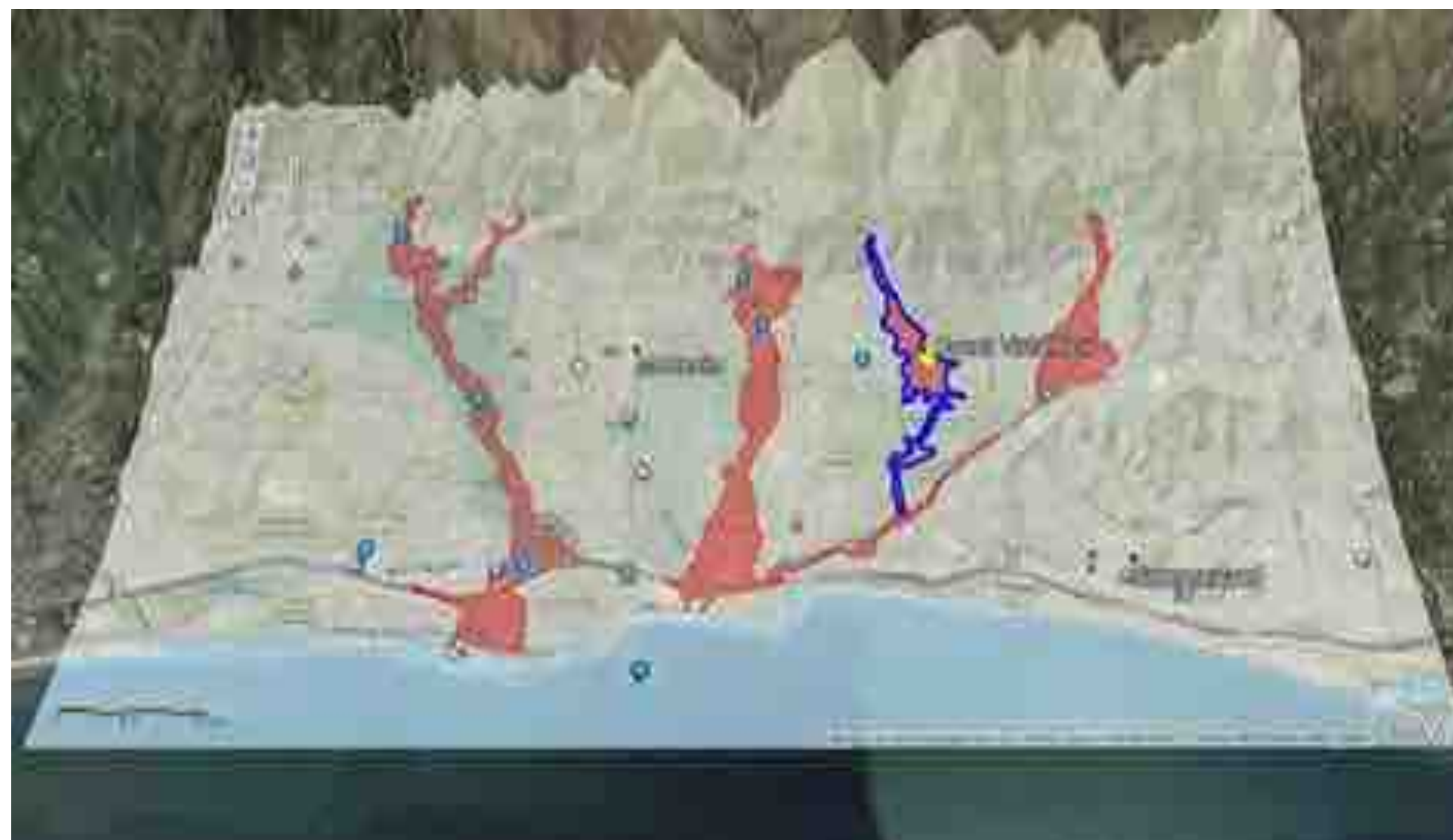
Buena Vista Creek is a small watershed that originates in the foot of the Santa Ynez Mountains and drains a 1,472-acre area capable of producing 2,800 cfs during a 100 year storm event. Buena Vista Creek is characterized by dry, rocky substrate and steep, deep banks with residential lawns and open space immediately adjacent to the top of both banks.
