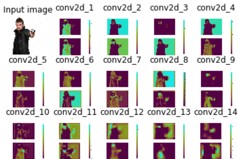
Fig. 5. Two activation map/filters layer by layer.
