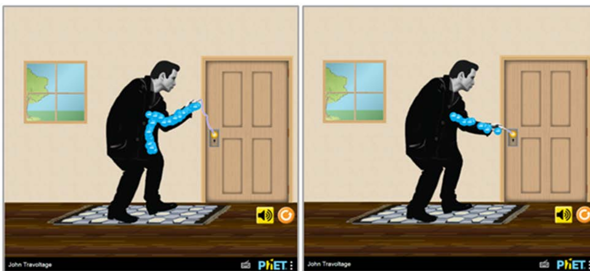
Fig. 1. Screenshot of PhET sim John Travoltage. Left panel: Hand away from doorknob, many charges have built up before discharge, discharge occurring. Right panel: Hand near doorknob, few charges have built up before discharge, discharge occurring
